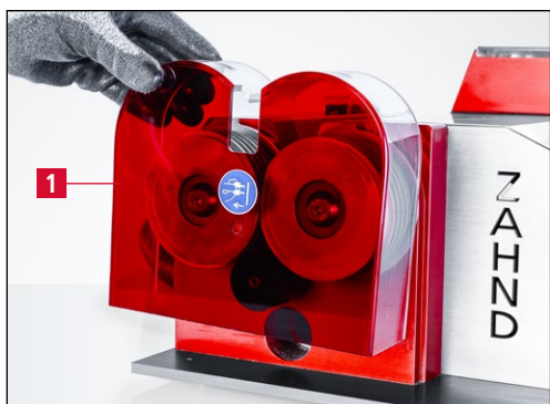
Figure 7-7 Retirer le capot de protection
