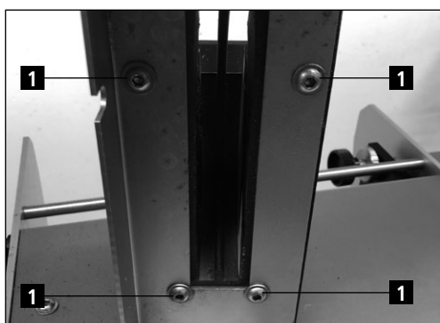
Figure 1-15 Ajuster le capot
