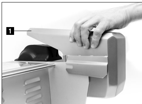
Figure 1-13 Retirer le capot antiprojections
