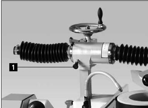
Figure 7-8 Desserrer la fixation
